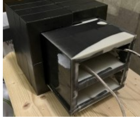
Fig. 7. The proposed transformer with plastic molding only in the electric field concentration area.
