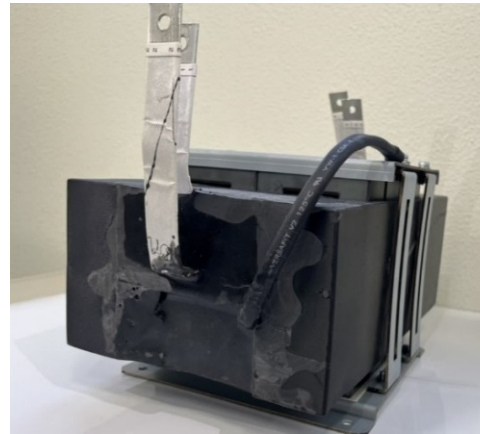
Fig. 8. The conventional transformer with plastic molding over entire winding.
