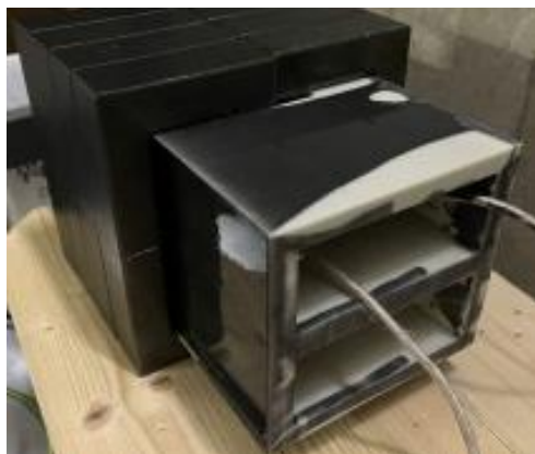
Fig. 6. Transformer molded only in the electric field concentration area.
