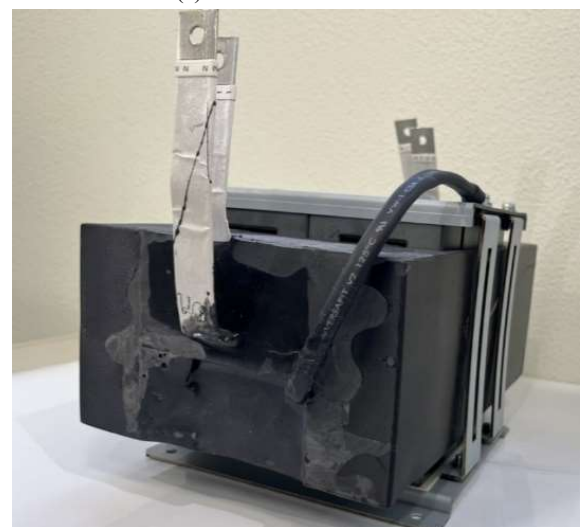
(b) Molded transformer.
