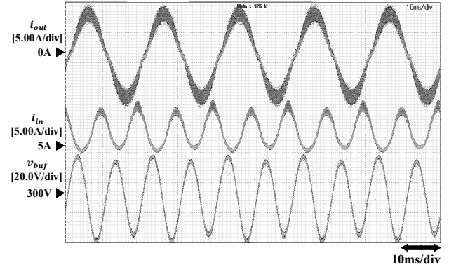
Fig.2 Experimental results of comparative circuit (output current, input current, capacitor voltage)
