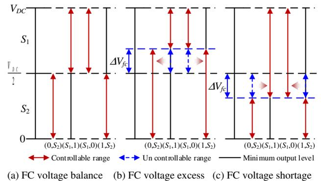
Fig. 6. Controllable range of output voltage of 2-series FCLA.
