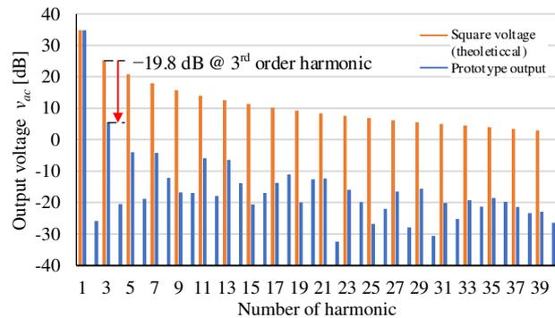
Fig. 12. Harmonic analysis of unfolder output voltage.
