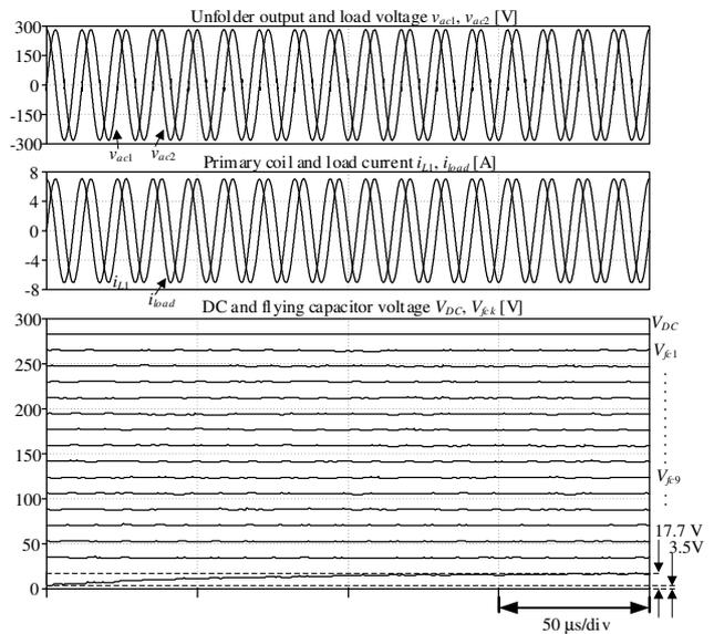
Fig. 8. Simulation waveform when the FC voltage unbalanced
