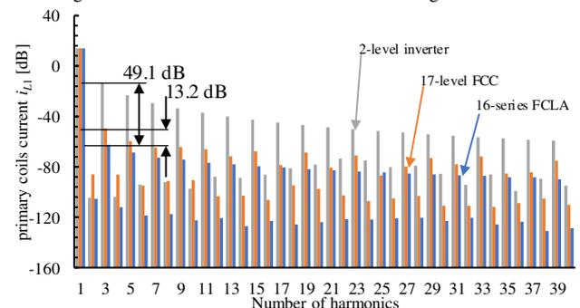
Fig. 9. Harmonic analysis for primary coil current
