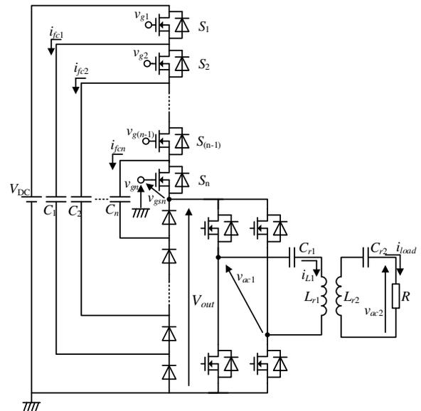
Fig. 2. FCLA with the unfold for WPT.
